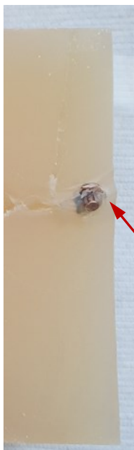
Figure 22: The bullet path must be recorded up to the outer edge of the bullet (see arrow).
